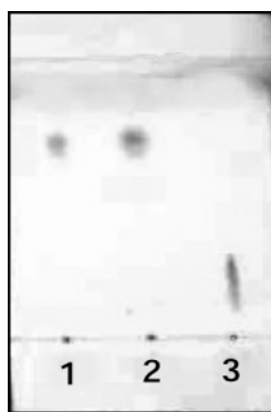
Fig. 3. TLC analysis of the Sommelet reaction product from Lac-NH 2 . Samples were visualized with methanol–sulfuric acid. Lane 1, reaction mixture; lane 2, lactose; lane 3, Lac-NH 2 .
